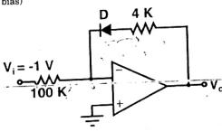
For an input voltage  $V_{_{\rm T}}$  = -I V, the output voltage  $V_{_{\rm 0}}$  is
