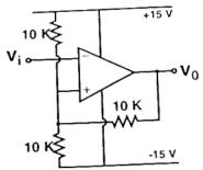
A triangular wave which goes from -12 V to 12 V is applied to the inverting input of the OPAMP. Assume that the output of the OPAMP swings from +15V to -15V. The voltage at the non-inverting input switches between
