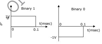
The source output is transmitted using two modulation schemes, namely Binary PSK (BPSK) and Quadrature PSK (QPSK). Let  $B_1$  and  $B_2$  be the bandwidth requirements of BPSK and QPSK respectively. Assuming that the bandwidth of the above rectangular pulses is 10 kHz,  $B_1$  and  $B_2$  are
