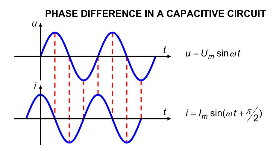
There is a **phase difference** between voltage and current Current is ahead of voltage (current leads voltage) Voltage is delayed as to current (voltage lags current)
