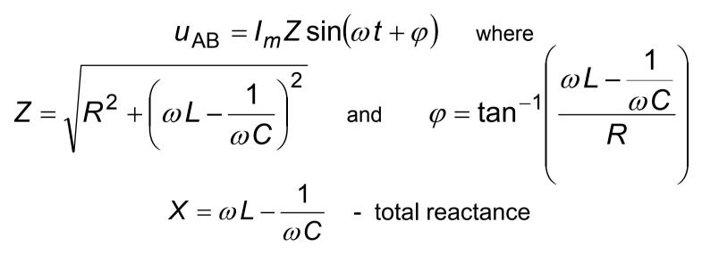
$\varphi$  - phase difference between voltage and current
