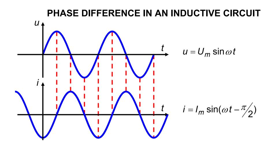
There is a **phase difference** between voltage and current Current is behind voltage (current lags voltage) Voltage is ahead of current (voltage leads current)
