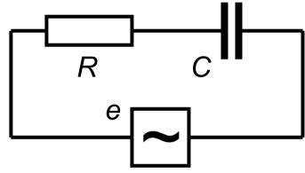
$U_{R} = IR : U_{R} \text{ in-phase with } I$  $U_{C} = IX_{C} : U_{L} \text{ lags } I \text{ by } \pi/2$  $X_{C} = \frac{1}{\omega C}$
