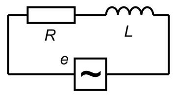
$U_R = IR$  :  $U_R$  in-phase with I $U_L = IX_L$  :  $U_L$  leads I by  $\pi/2$  $X_L = \omega L$
