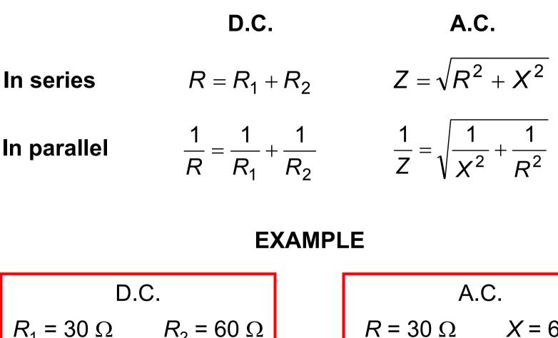
D.C.  $R_1 = 30 \Omega$   $R_2 = 60 \Omega$ in parallel  $R = 20 \Omega$ (33% less than  $R_1$ ) A.C.  $R = 30 \Omega$   $X = 60 \Omega$ in parallel  $Z = 26.8 \Omega$ (10% less than R)
