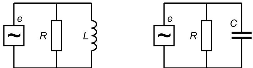
CR or LR circuits in parallel. How to analyse them using phasor diagrams?
