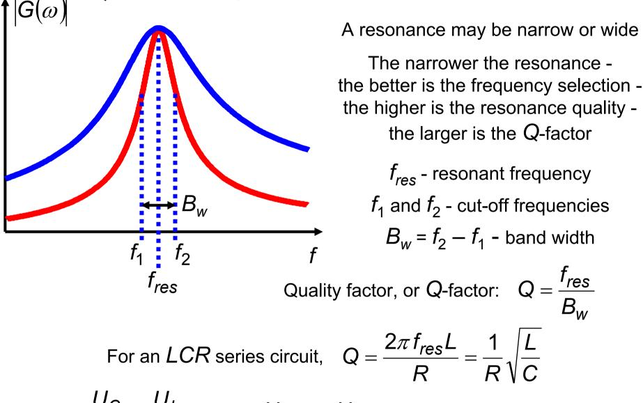
Also,  $Q = \frac{U_C}{U_{in}} = \frac{U_L}{U_{in}}$  where  $U_C$  and  $U_L$  are voltages across the capacitor and the inductor at the resonance, respectively
